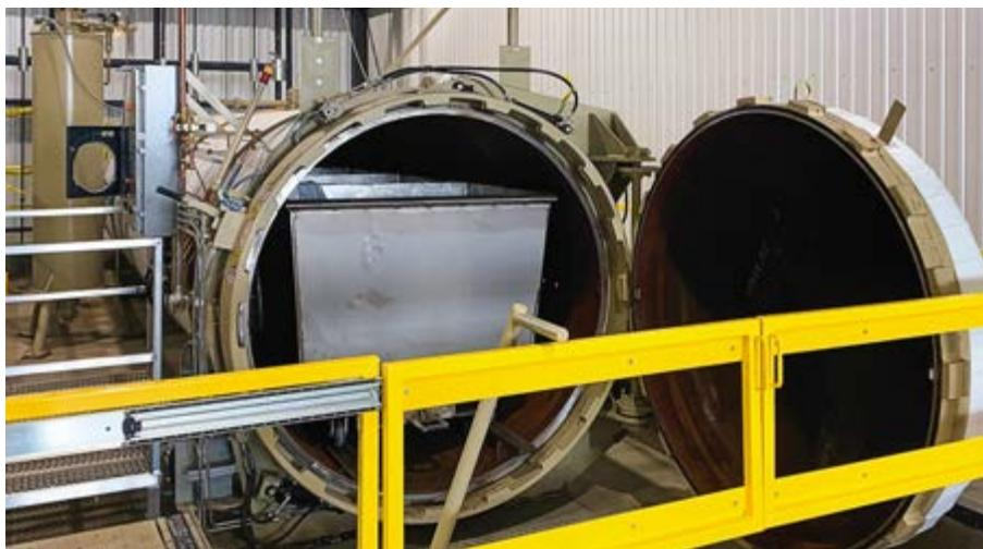
The large stainless steel bins enter the autoclave for the one-hour sterilization process.
